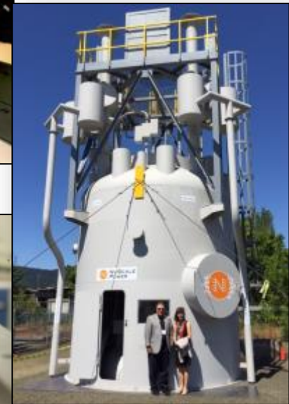
NuScale Full-scale Upper Module Mockup
