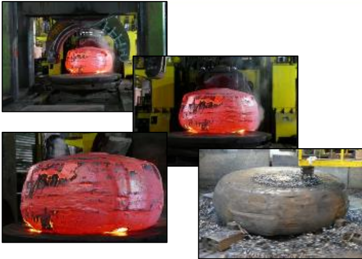
NuScale RPV Head Ingot Being Forged
